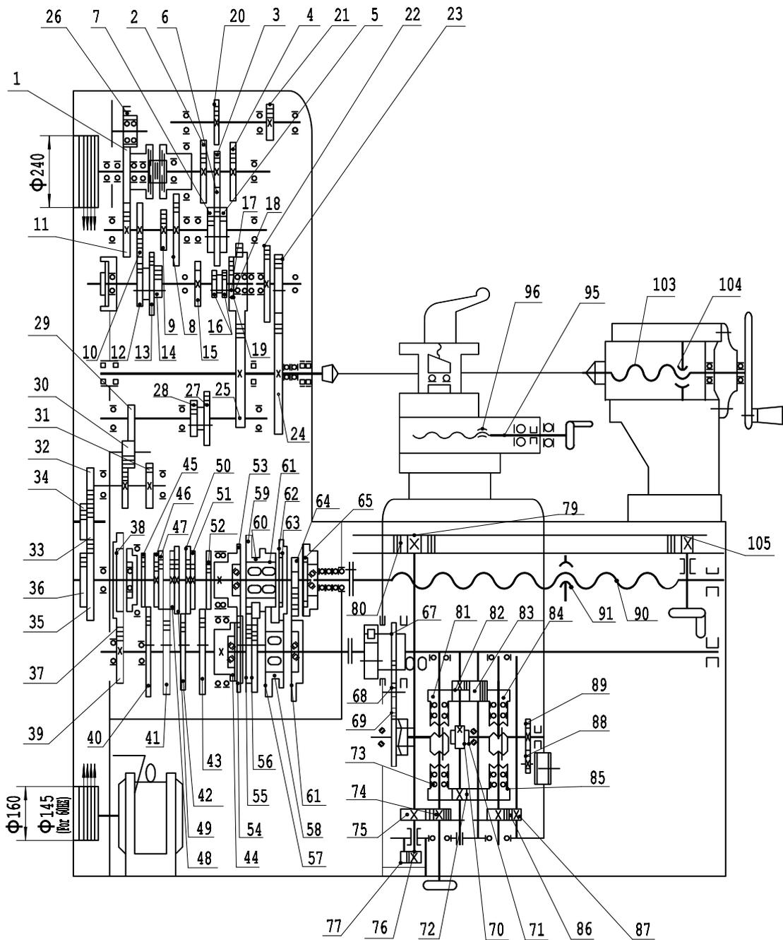
Fig. 19 Arrangement of rolling bearings for CW63C, CW93C
