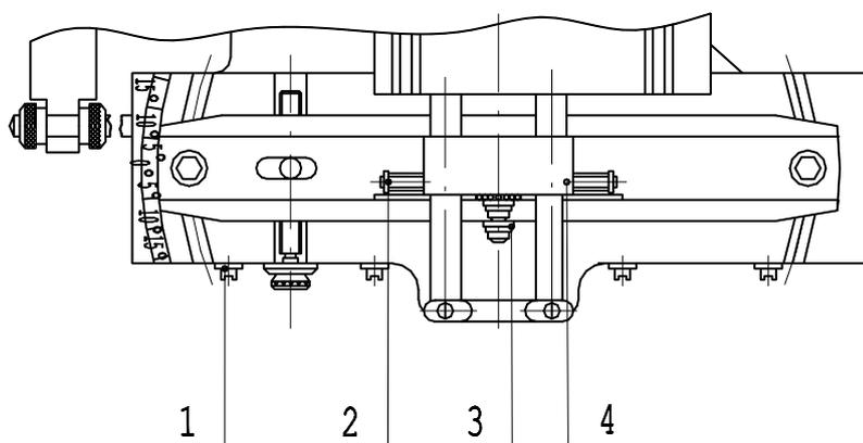
Fig. 47 Adjustment of taper attachment
