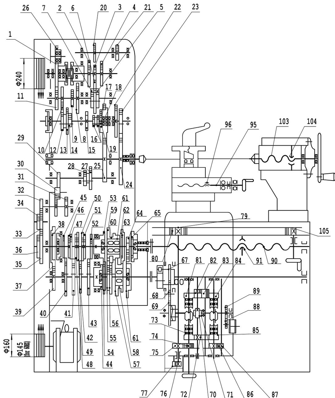
Fig. 15 Driving system diagram for CW63B series and CW93B series
