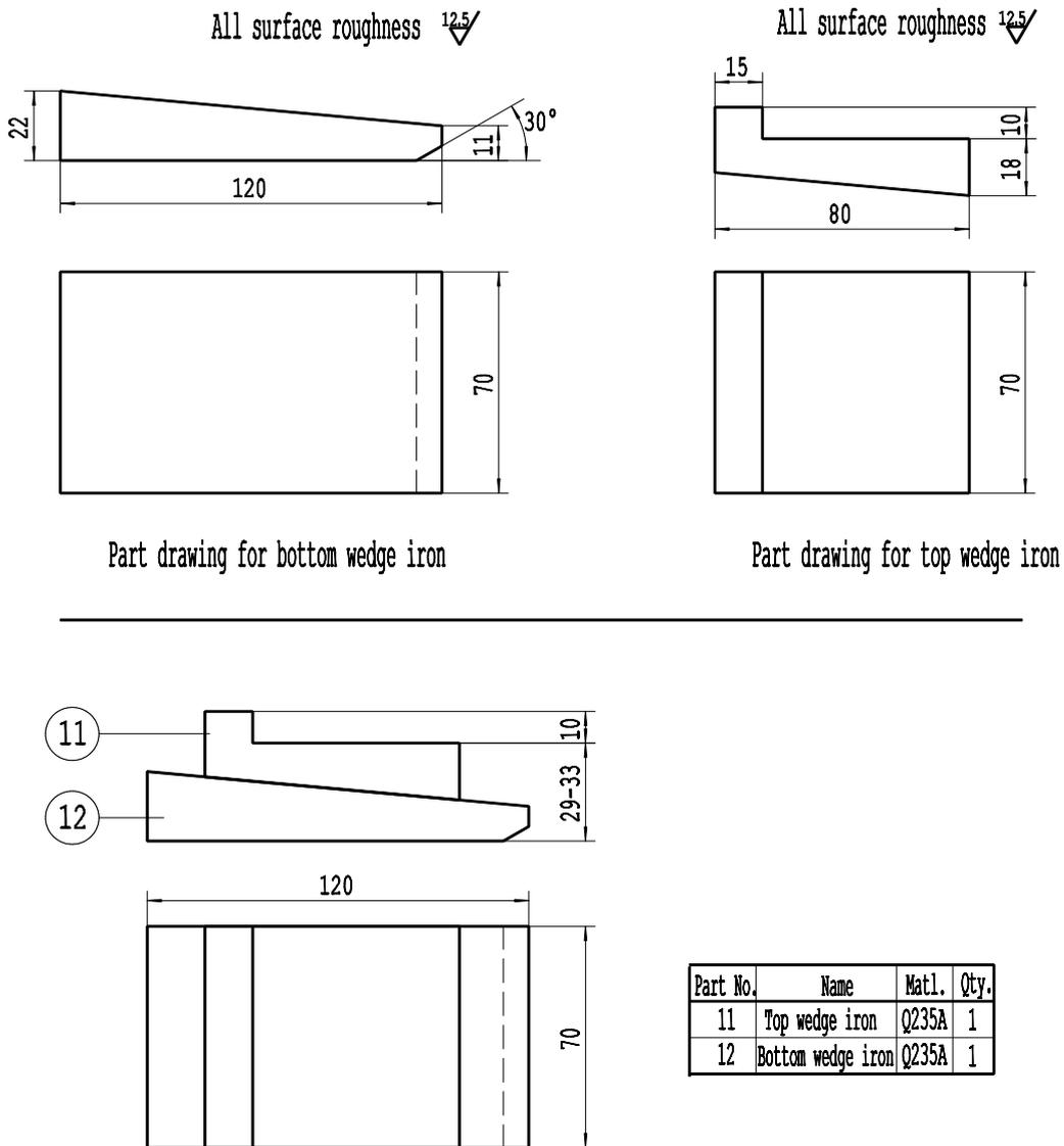
Fig. 2 Part drawing for wedge irons
