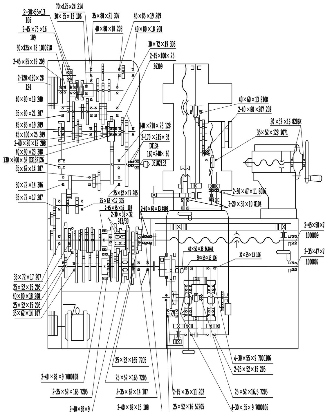
Fig. 18 Arrangement of rolling bearings for CW63B and CW93B
