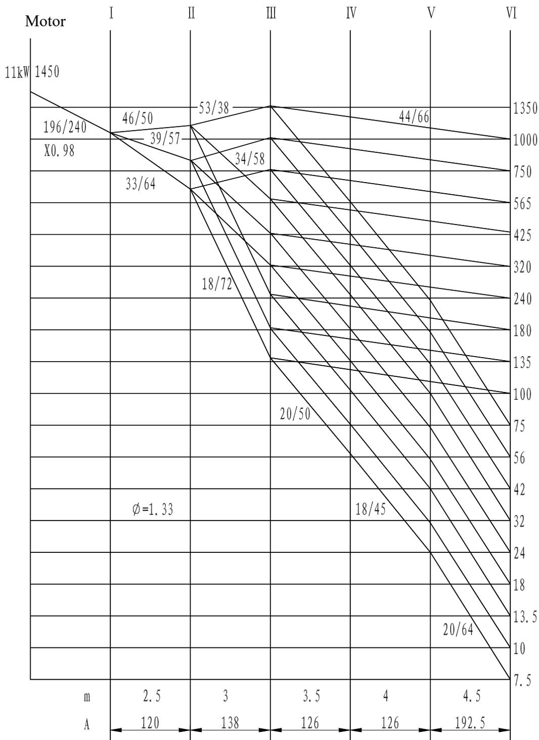
Fig. 16 Distributing diagram of speed for CW63B
