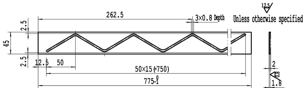
This part will bind with 16C05011 and the oil groove will be machined.
