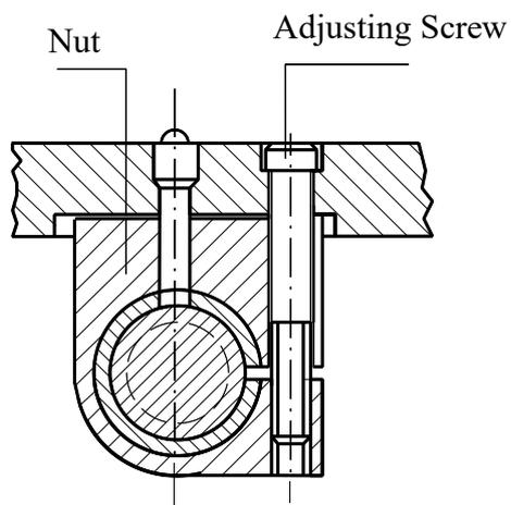
Fig. 46 Adjustment of Leadscrew for Carriage
