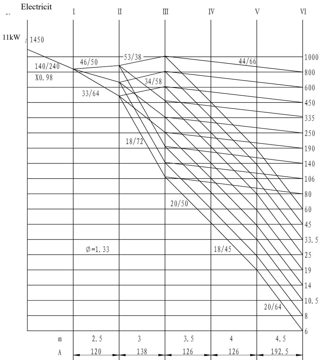
Fig. 21 Distributing Diagram of Speed for CW93C
