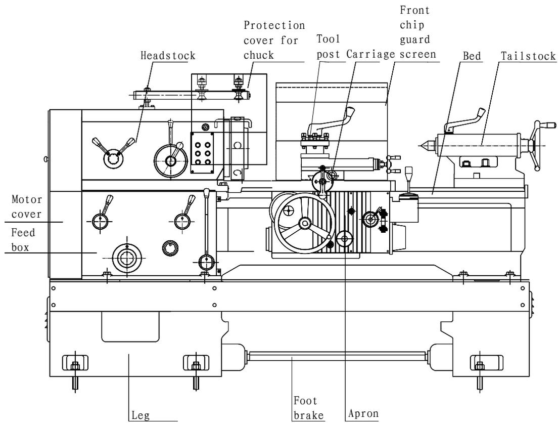
Fig. 12 Appearance view of the machine with foot-pedal braking
