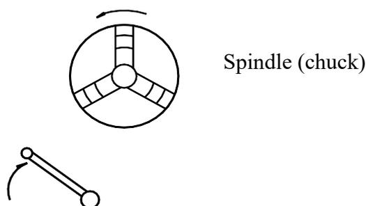
Fig. 27 Operating handle for forward and reverse of spindle and rotating direction of spindle
