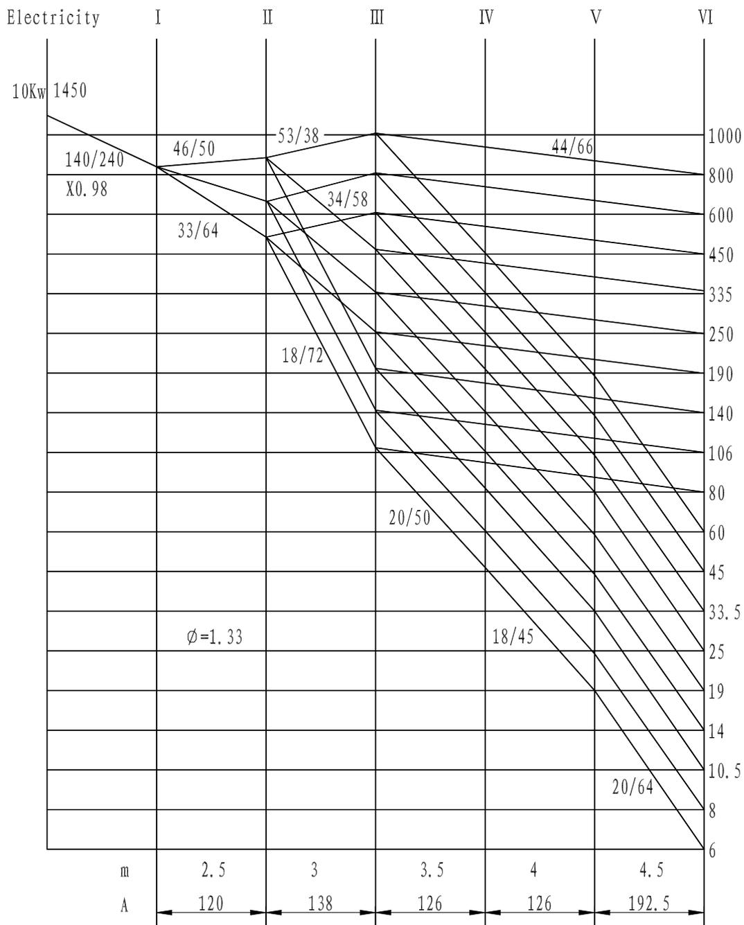
Fig. 17 Distributing diagram of speed for CW93B
