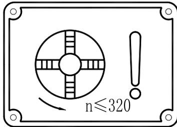
Fig. 75 Limit speed label of 4-jaw chuck
