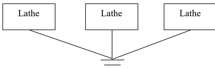
Never connect to one grounding rod for some equipment like the figure given below:
