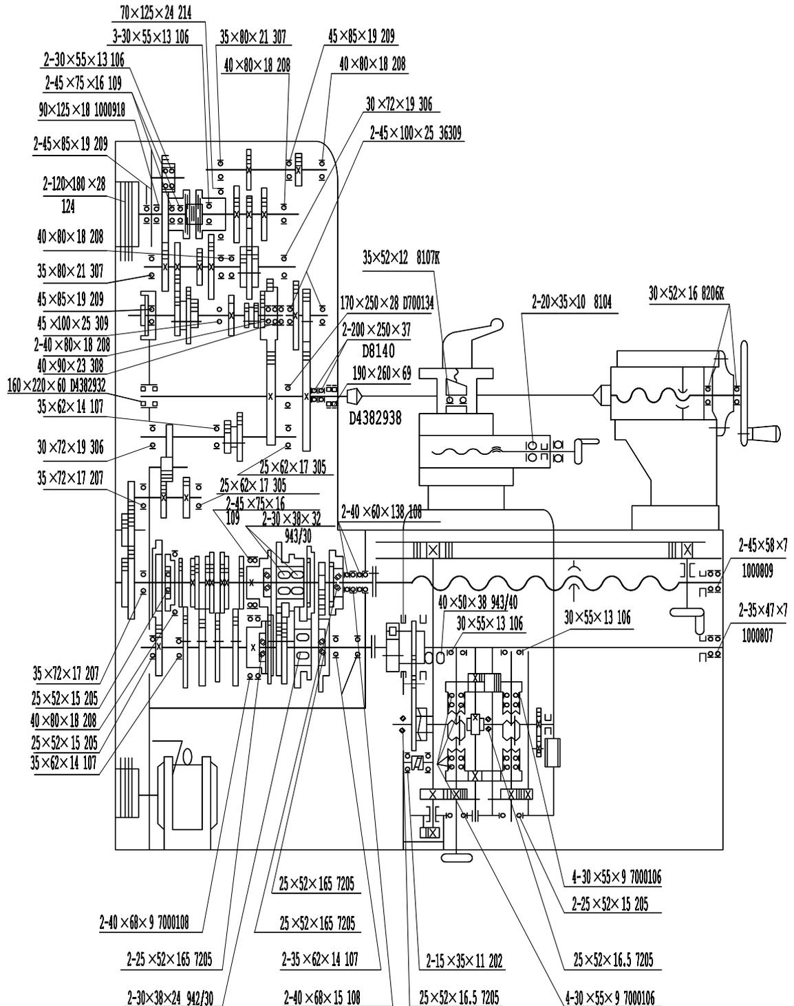
Fig. 22 Arrangement of Roller Bearings of CW63C and CW93C
