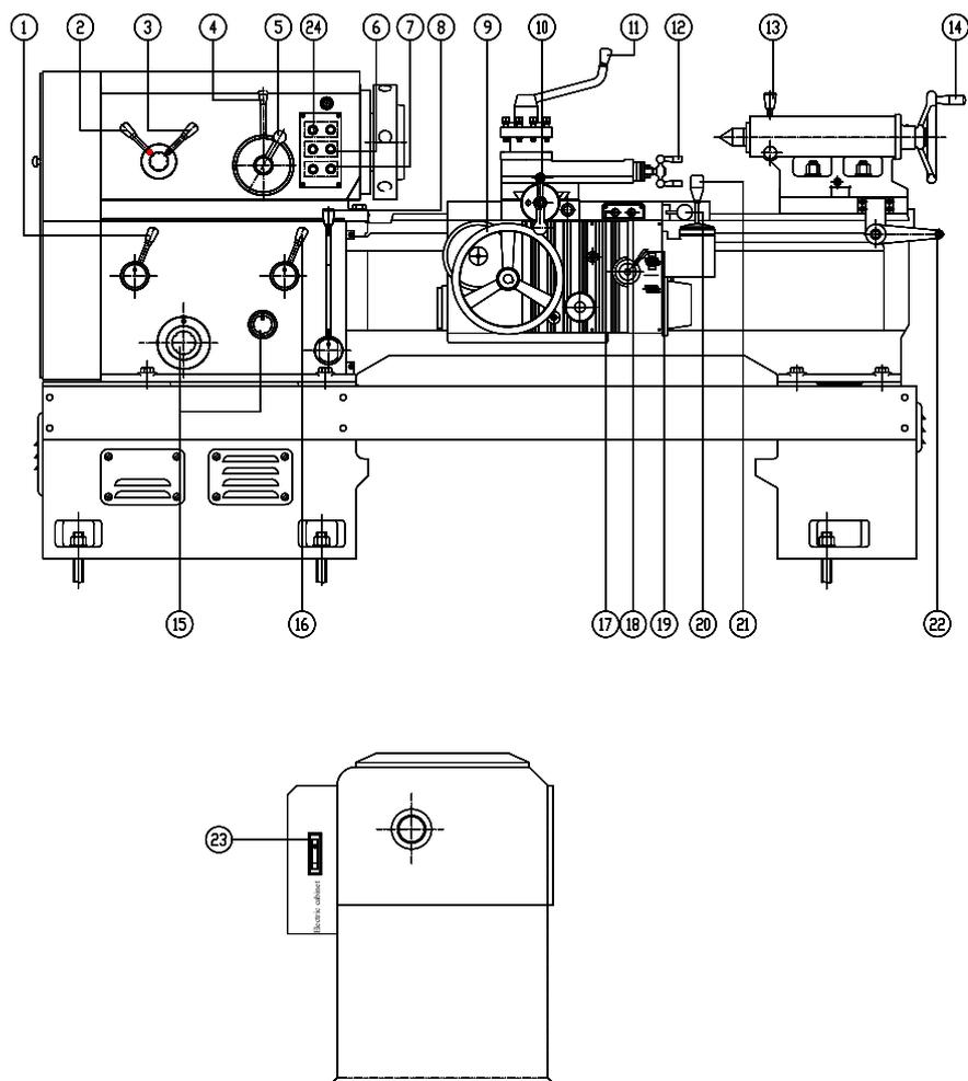
Fig. 23 Control levers of the machine with hand-braking
