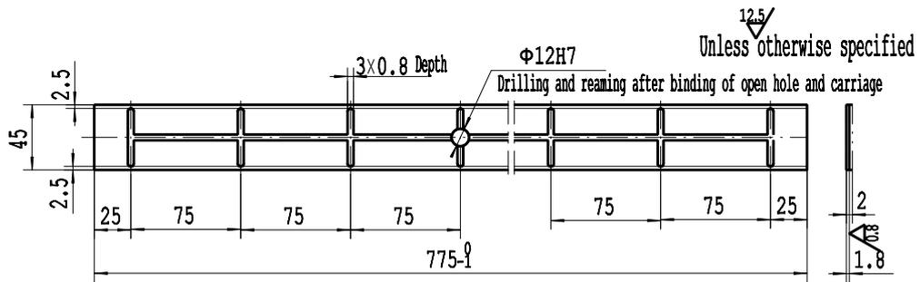
This part will bind with 16C05011 and the oil groove will be machined.
