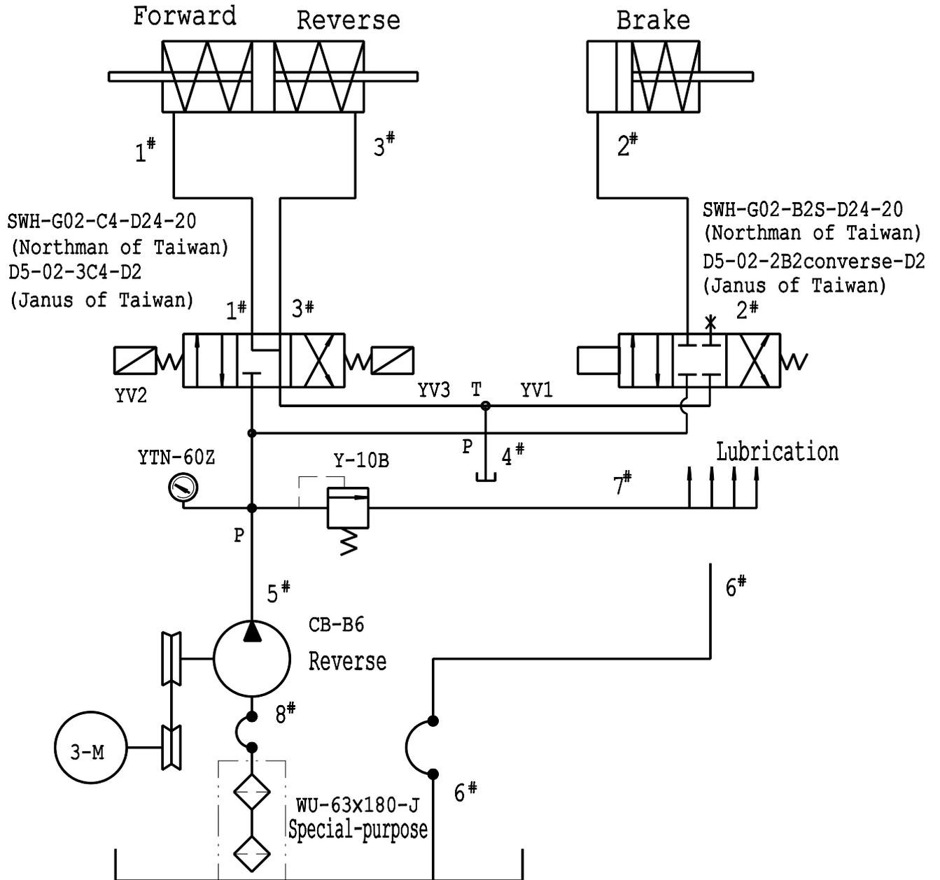
Fig. 14 Hydraulic principle diagram for the machine of 4m or more than 4m
