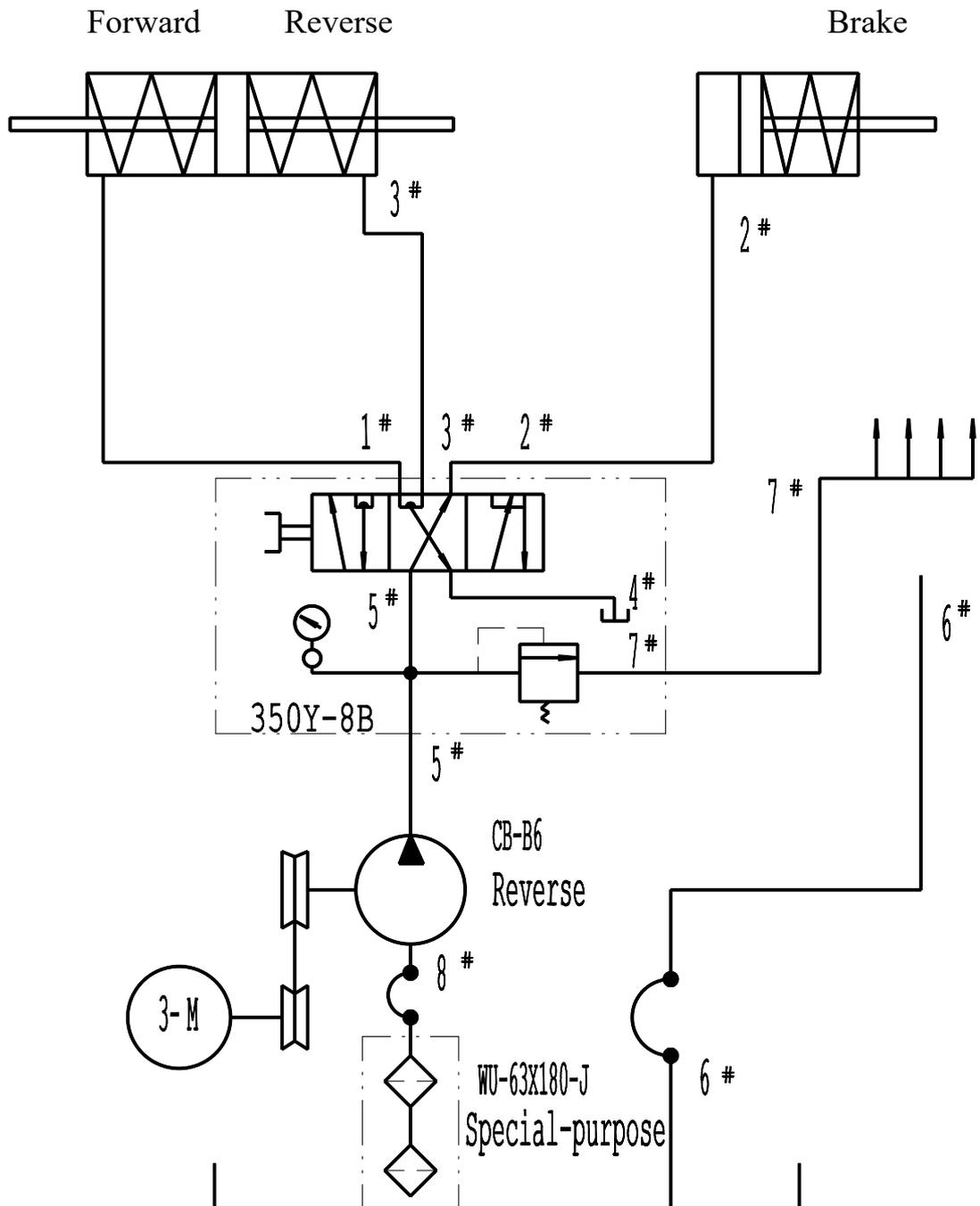
Fig.13 Hydraulic principle diagram for the machine of 3m or less than 3m
