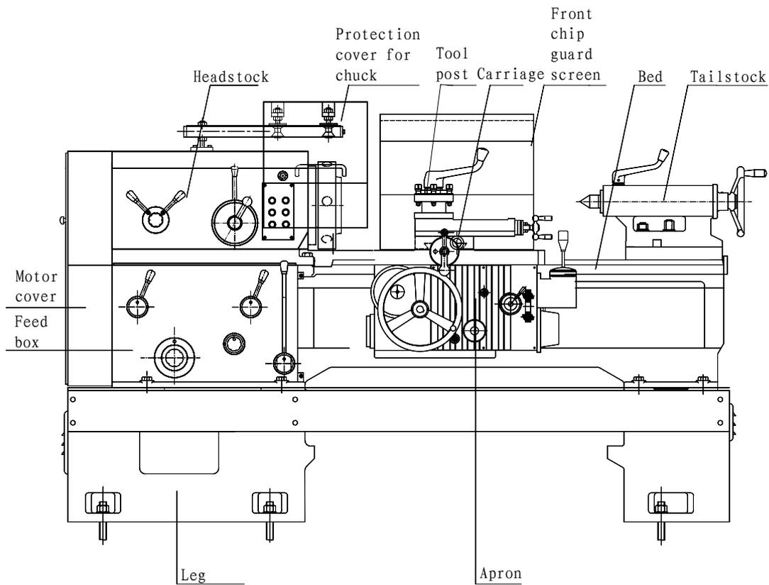
Fig. 11 Appearance view of the machine with hand-brake
