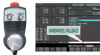
Handwheel forward → program forward execution Handwheel reversal → program reversal execution
