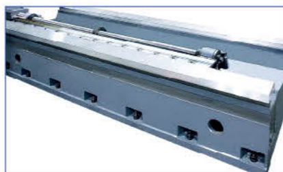
Bed column adopts integral steel guiderail which features quenching grinding and hardness of HRC60±2.
