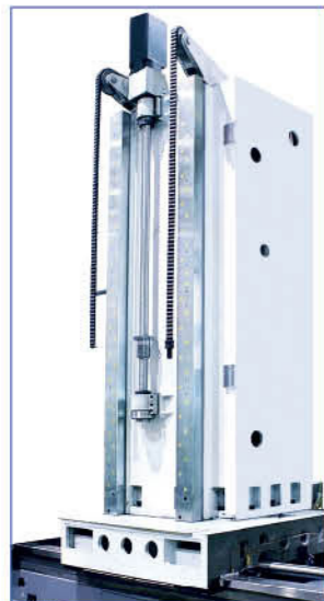
Bed column adopts integral steel guiderail which features quenching grinding and hardness of HRC60±2.
