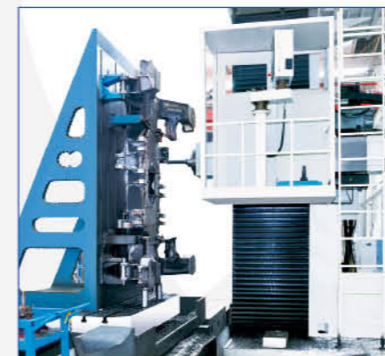
Machining by using bent plate
