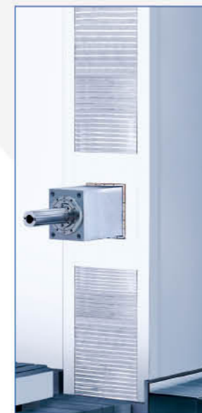
Armor protection of column
