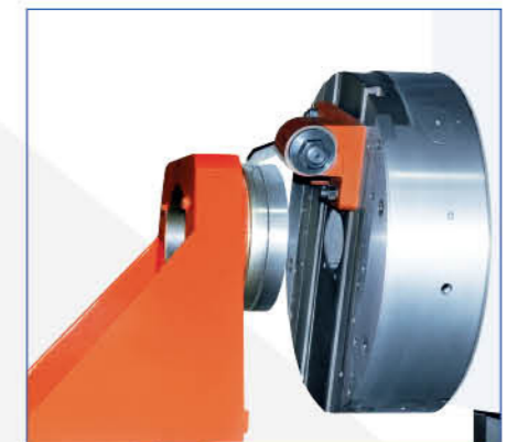
Machining by using facing head
